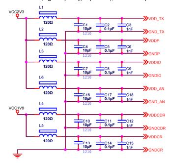
FIGURE 5. POWER SUPPLY BYPASSING
