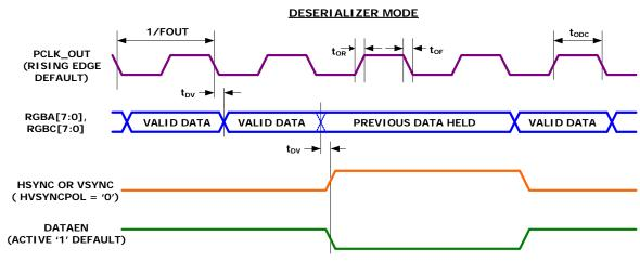
FIGURE 4. PARALLEL VIDEO OUTPUT TIMING
