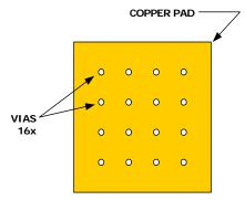
FIGURE 6. LAYOUT FOR THE EXPOSED PAD
