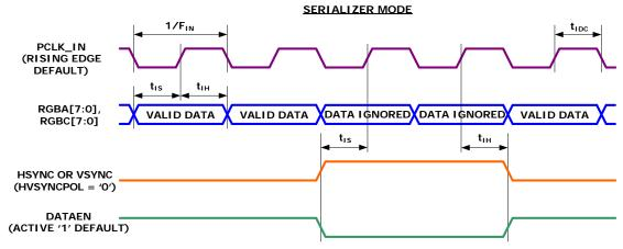
FIGURE 3. PARALLEL VIDEO INPUT TIMING
