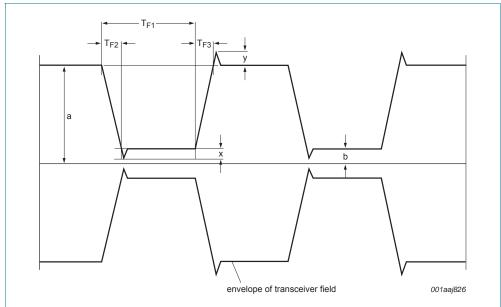
Fig 6. Modulation details of data transmission from RWD to HITAG  $\mu$  transponder IC
