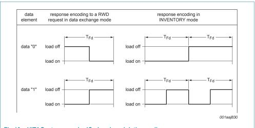
Fig 10. HITAG μ transponder IC - Load modulation coding
