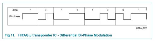
Differential Bi-phase (or FM0 respectively) contains a transition in the center of bit conversion representing Data '0' and no one for Data '1'. At the beginning of every bit modulation a level transition must be performed.
