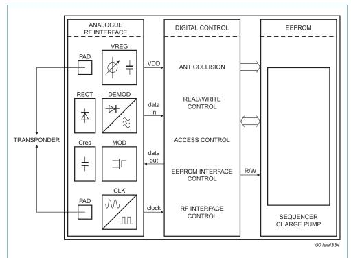
Fig 1. Block diagram of HITAG μ transponder IC
