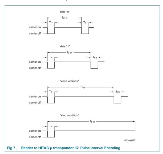
Assuming equal distributed data bits '0' and '1', the data rate is in the range of about 5.2 kbit/s.
