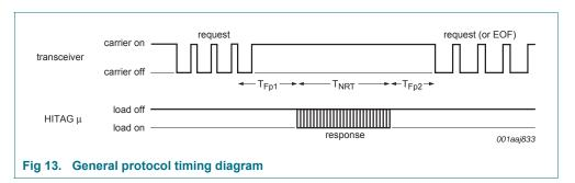
The minimum value of  $T_{Ep1}$  is  $T_{Ep1min} = 204 \times T_{C}$
