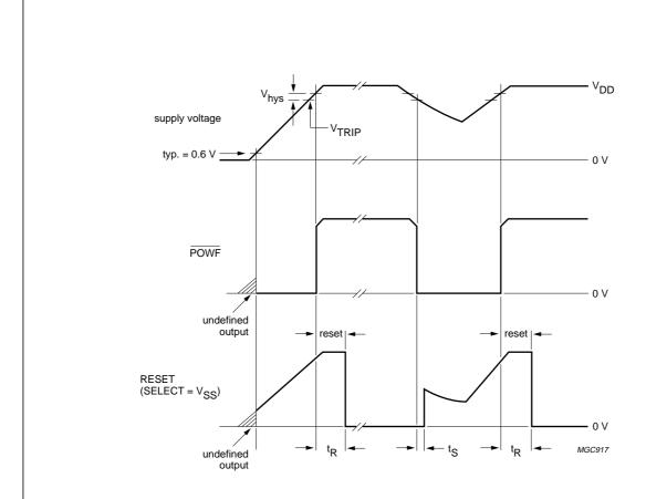
$t_R$  = reset time (duration of reset pulse).
