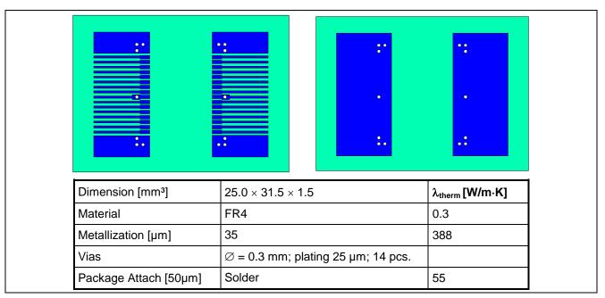
Figure 17 PCB reference layout (left: top layer, right: bottom layer)
