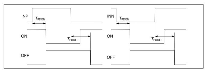
Figure 7 Timing of turn-on and turn-off propagation delay without two-level turn-off mode
