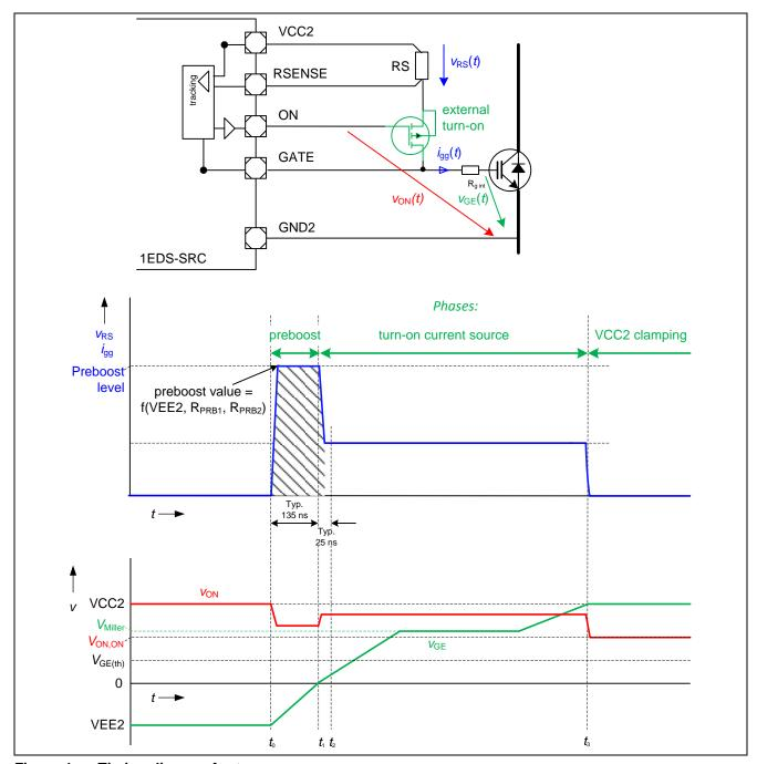
Figure 4 Timing diagram for turn-on
