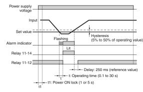
Note: The power ON lock prevents unnecessary alarms from being generated during the instable period when the power is first turned on. There is no relay output during timer operation.
