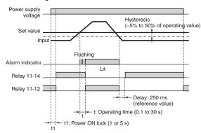
Note: The power ON lock prevents unnecessary alarms from being generated during the instable period when the power is first turned on. There is no relay output during timer operation.
