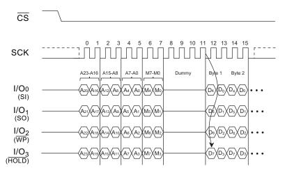
Figure 6-8. Quad I/O Read Array with Continuous Read Mode (Previous Command Set M5-4 =1,0)
