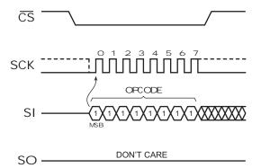
Figure 6-10. Continuous Read Mode Reset (Dual)
