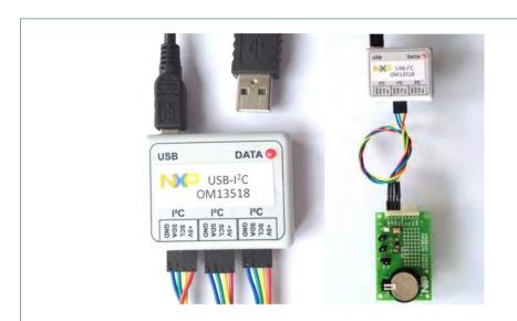
Fig 4. A) Dongle OM13518, B) connected to the evaluation board OM13514
