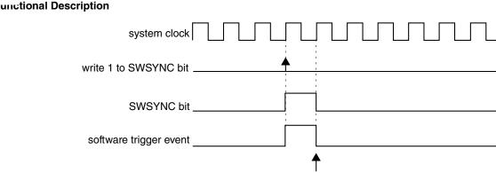
FTM counter is reset and channel outputs are forced to their initial value
