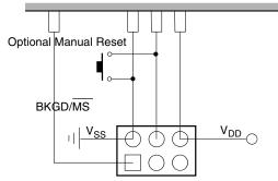
Figure 2-8. Typical debug circuit
