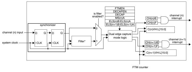
\* Filtering function for dual edge capture mode is only available in the channels 0 and 2
