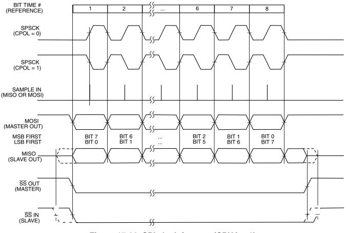
Figure 17-26. SPI clock formats (CPHA = 0)
