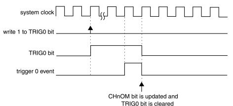
Figure 12-232. CHnOM synchronization when (SYNCHOM = 1), (PWMSYNC = 0), and a hardware trigger was used
