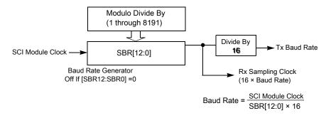
Figure 15-35. SCI baud rate generation
