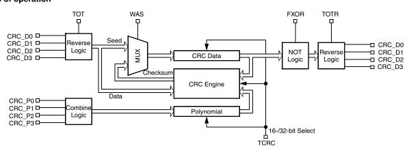
Figure 21-1. Cyclic redundancy check (S08CRC) block diagram
