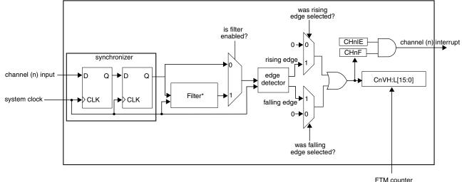
\* NOTE: Filtering function is only available in the inputs of channel 0, 1, 2, and 3
