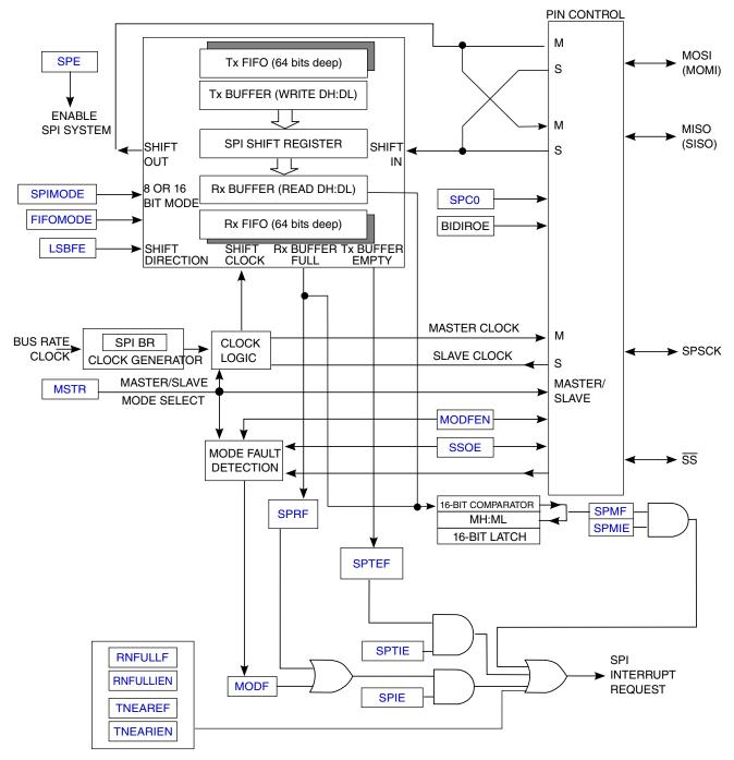
Figure 17-2. SPI Module Block Diagram with FIFO
