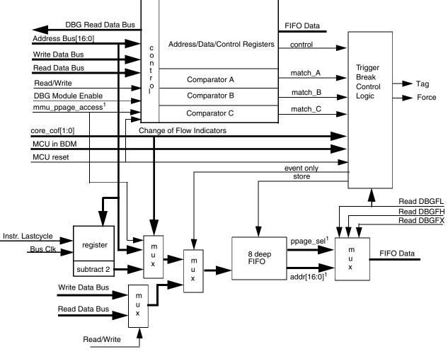
Figure 24-1. DBG block diagram
