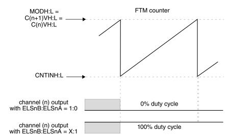
Figure 12-214. Channel (n) output if (C(n)V = C(n+1)V = MOD)
