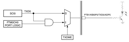
Figure 6-2. IR modulation diagram
