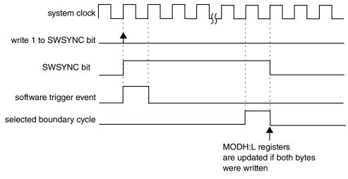
Figure 12-229. MODH:L synchronization when (PWMSYNC = 1)
