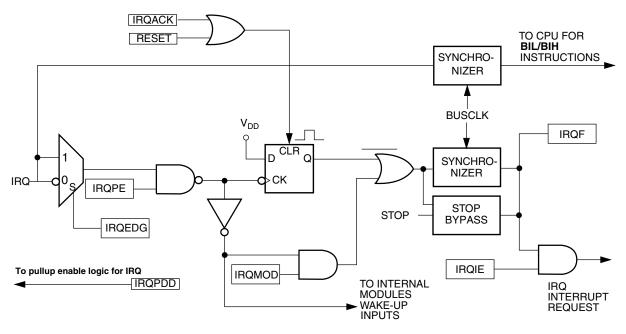
Figure 5-3. IRQ module block diagram
