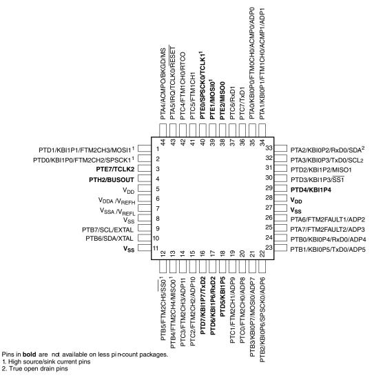
Figure 2-3. MC9S08PA60 44-pin LQFP package
