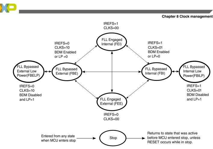
Figure 8-3. ICS clocking switching modes
