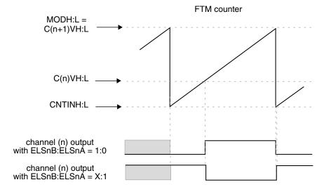
Figure 12-207. Channel (n) output if (CNTIN < C(n)V < MOD) and (C(n+1)V = MOD)
