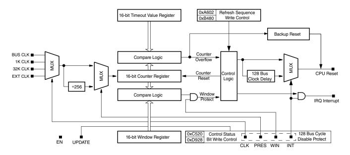
Figure 22-1. WDOG block diagram
