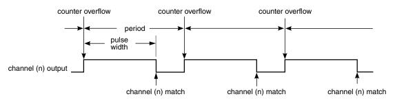
Figure 12-199. EPWM period and pulse width with ELSnB:ELSnA = 1:0
