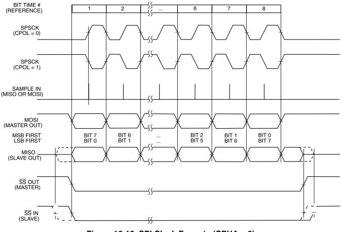
Figure 16-16. SPI Clock Formats (CPHA = 0)
