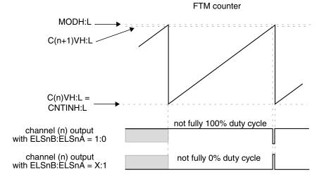
Figure 12-210. Channel (n) output if (C(n)V = CNTIN) and (CNTIN < C(n+1)V < MOD) and (C(n+1)V is almost equal to MOD)
