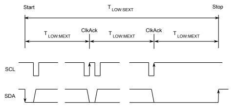
Figure 18-16. Timeout measurement intervals
