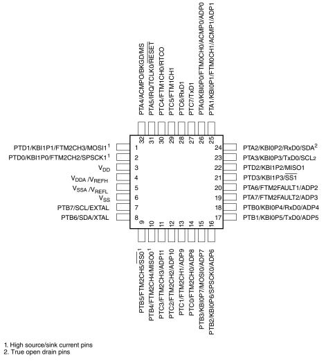
Figure 2-4. MC9S08PA60 32-pin LQFP package
