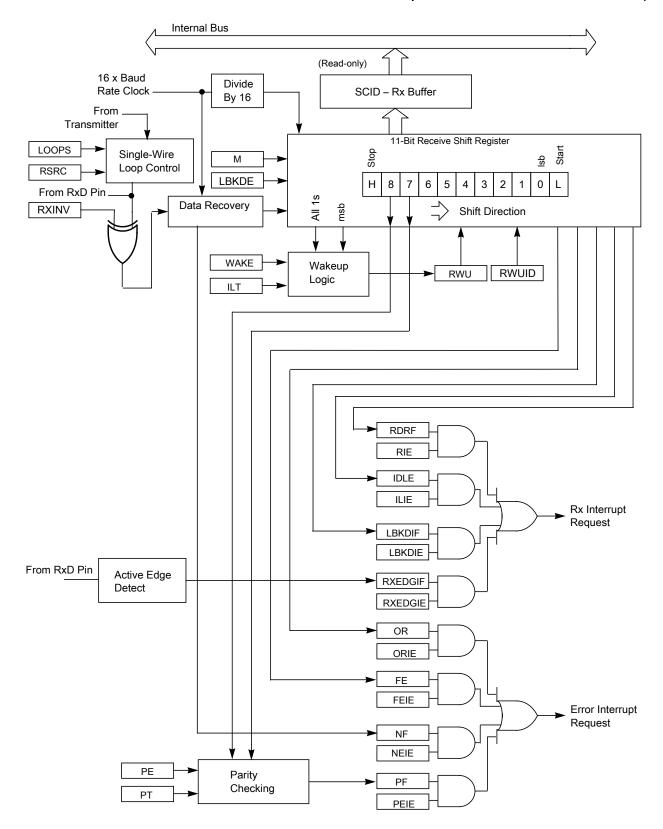
Figure 15-2. SCI receiver block diagram
