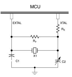
Figure 8-7. OSC high-gain mode connection
