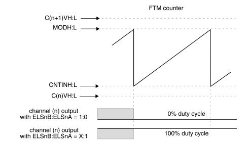
Figure 12-211. Channel (n) output if C(n)V and C(n+1)V are not between CNTIN and MOD
