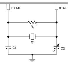
Figure 8-6. OSC low-power mode connection
