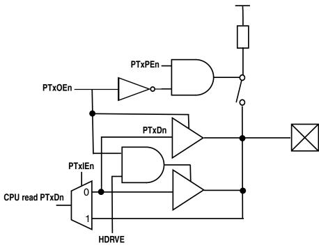
Figure 7-3. High drive I/O structure
