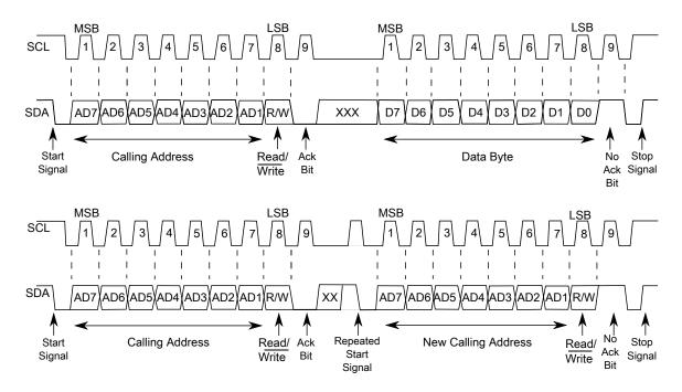
Figure 18-14. I2C bus transmission signals
