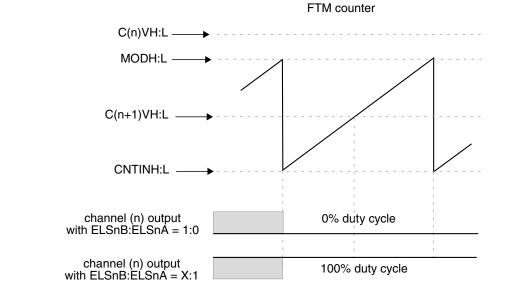
Figure 12-218. Channel (n) output if (C(n)V > MOD) and (CNTIN < C(n+1)V < MOD)
