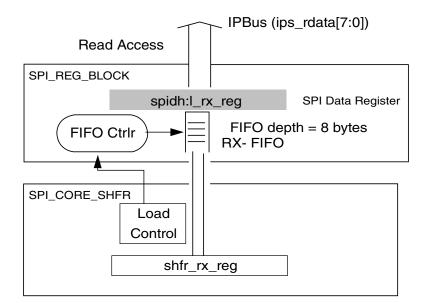
Figure 17-23. SPIH:L read side structural overview in FIFO mode
