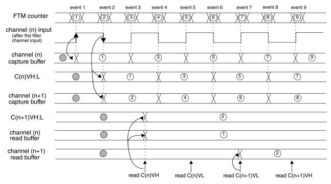
Figure 12-258. Dual edge capture mode read coherency mechanism
