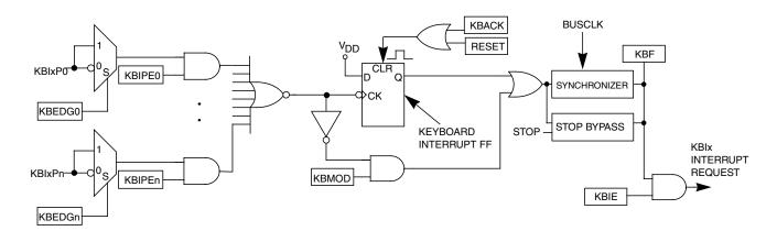
Figure 11-1. KBI block diagram
