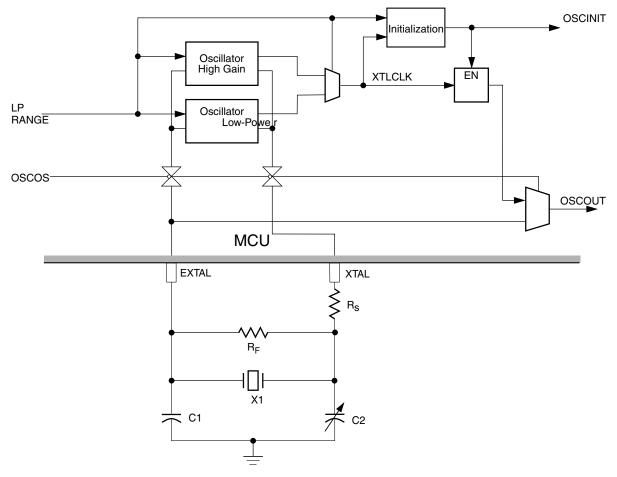
Figure 8-4. Oscillator module block diagram
