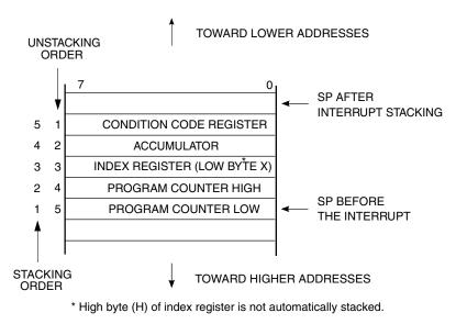
Figure 5-1. Interrupt stack frame
