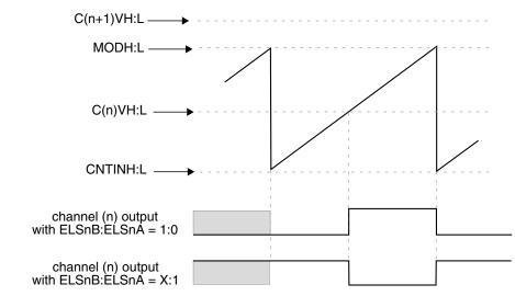
Figure 12-219. Channel (n) output if (C(n+1)V > MOD) and (CNTIN < C(n)V < MOD)
