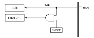
Figure 6-3. RxD0 capture function diagram
