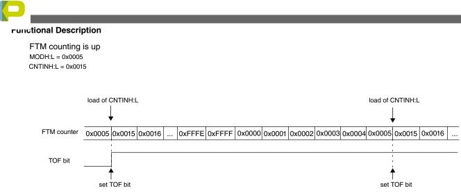
Figure 12-190. Example of up counting when the value of CNTIN registers is greater than the value of MOD registers
