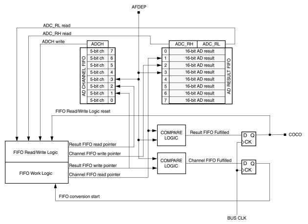
Figure 19-12. FADC FIFO structure
