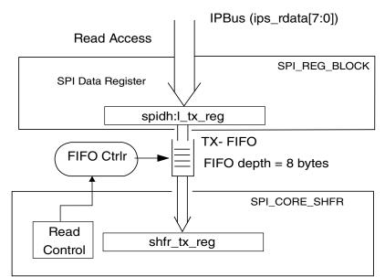
Figure 17-24. SPIH:L write side structural overview in FIFO mode
