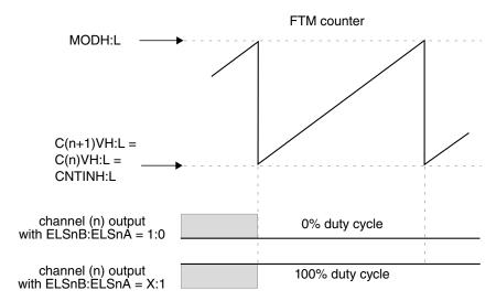
Figure 12-213. Channel (n) output if (C(n)V = C(n+1)V = CNTIN)
