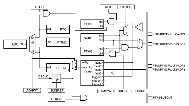
Figure 6-1. System interconnection diagram
