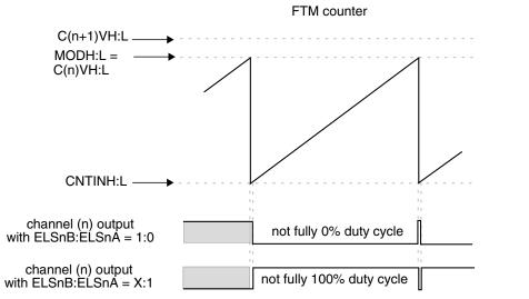
Figure 12-220. Channel (n) output if (C(n+1)V > MOD) and (CNTIN < C(n)V = MOD)
