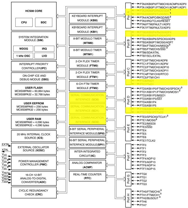
1. PTA2 and PTA3 operate as true open drain when working as output .
