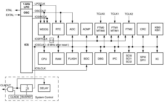
Figure 1-2. System clock distribution diagram
