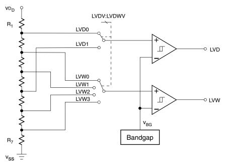
Figure 3-1. Low voltage detect (LVD) block diagram
