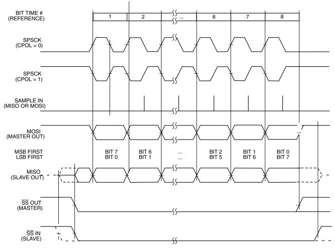
Figure 17-25. SPI clock formats (CPHA = 1)
