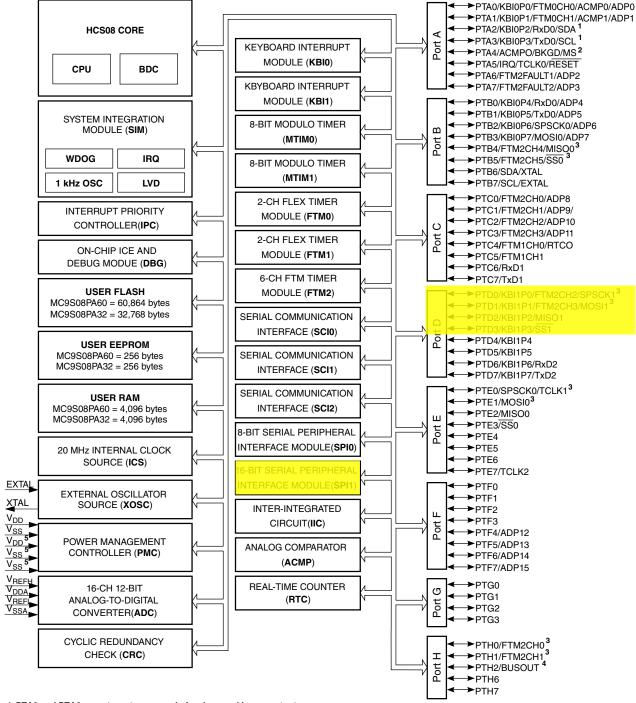
1. PTA2 and PTA3 operate as true open drain when working as output  $% \mathcal{A}$  .
