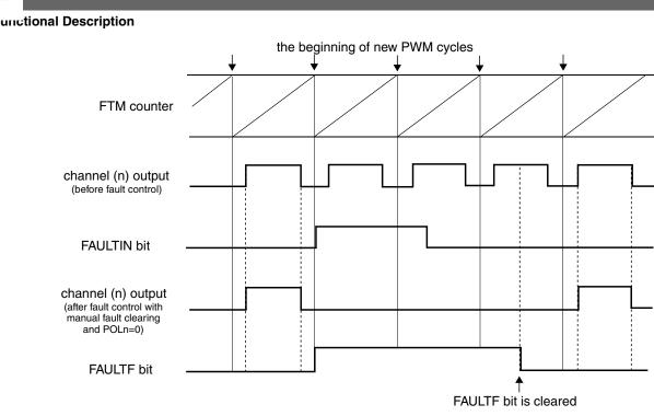
Figure 12-245. Fault control with manual fault clearing
