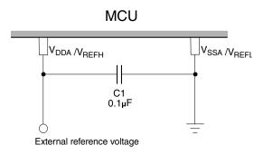
Figure 2-6. Analog power supply bypassing
