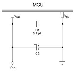
Figure 2-5. Power supply bypassing
