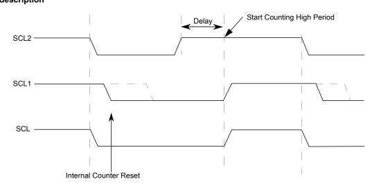
Figure 18-15. I2C clock synchronization
