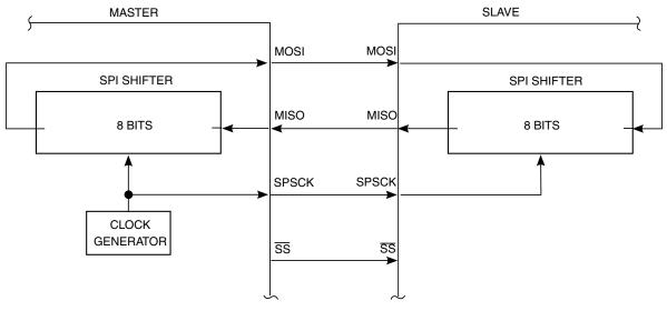
Figure 16-1. SPI System Connections
