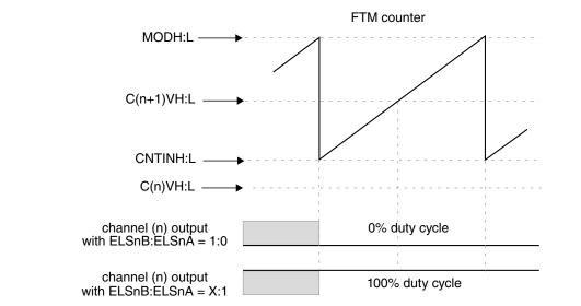
Figure 12-216. Channel (n) output if (C(n)V < CNTIN) and (CNTIN < C(n+1)V < MOD)
