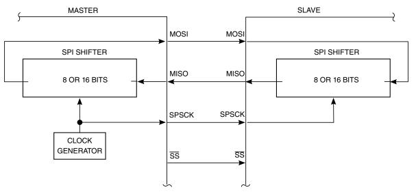
Figure 17-1. SPI system connections
