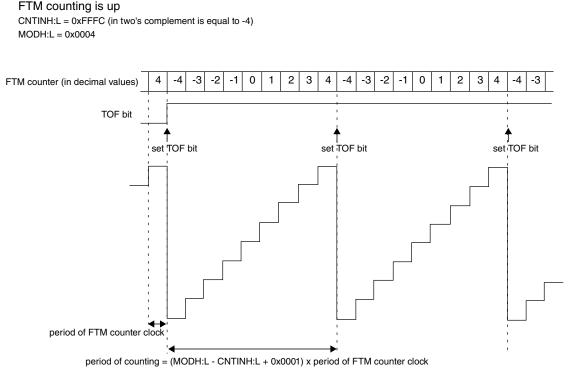
Figure 12-188. Example of FTM up and signed counting
