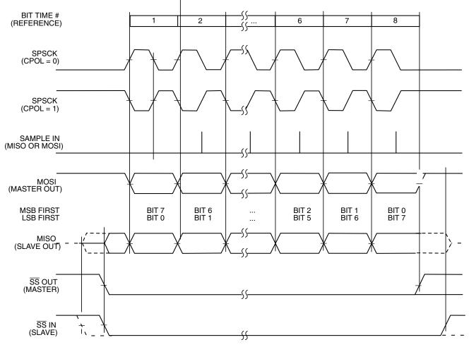
Figure 16-15. SPI Clock Formats (CPHA = 1)
