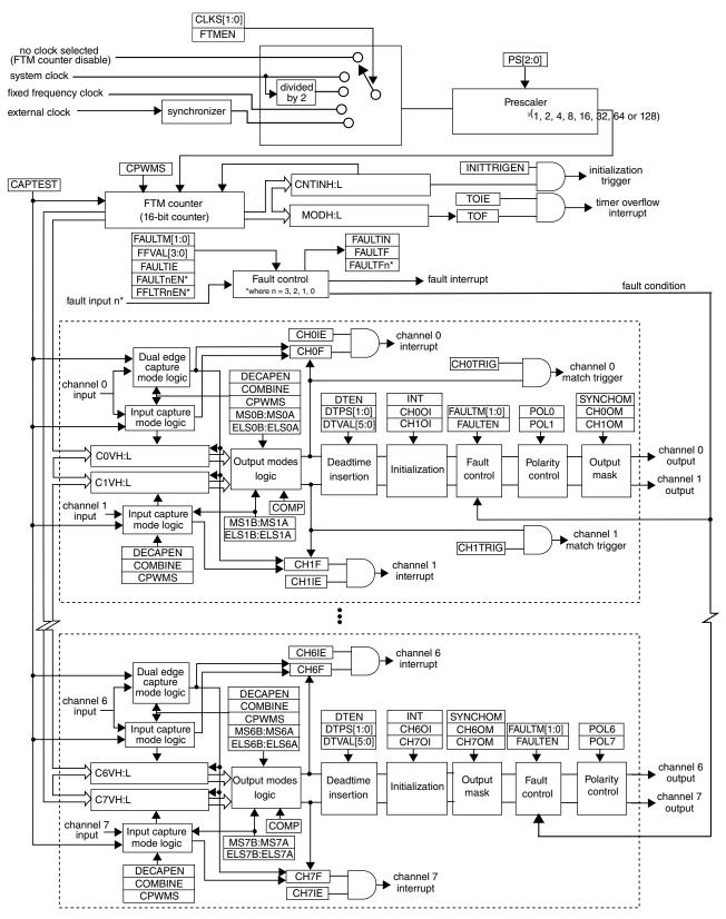
Figure 12-1. FTM block diagram
