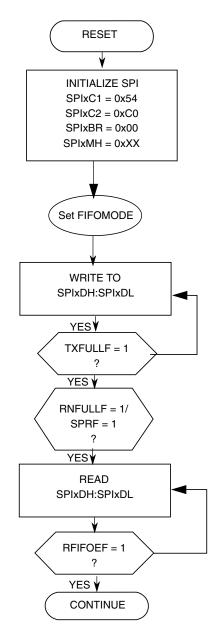
Figure 17-29. Initialization Flowchart Example for SPI Master Device in 16-bit Mode for FIFOMODE = 1
