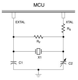
Figure 2-7. Typical crystal or resonator circuit
