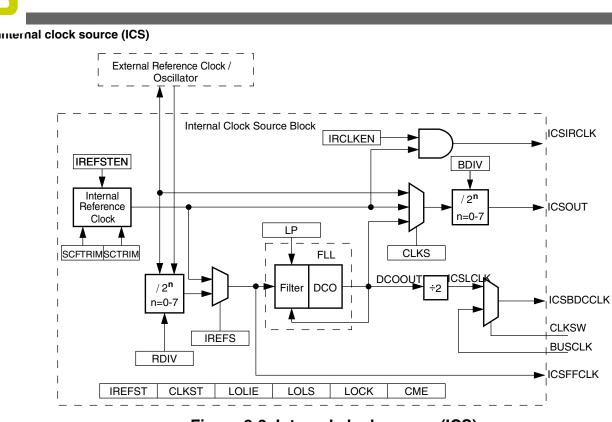
Figure 8-2. Internal clock source (ICS)
