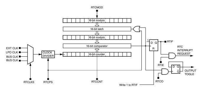
Figure 14-1. Real-time counter (RTC) block diagram
