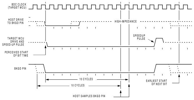
Figure 23-4. BDM target-to-host serial bit timing (logic 0)
