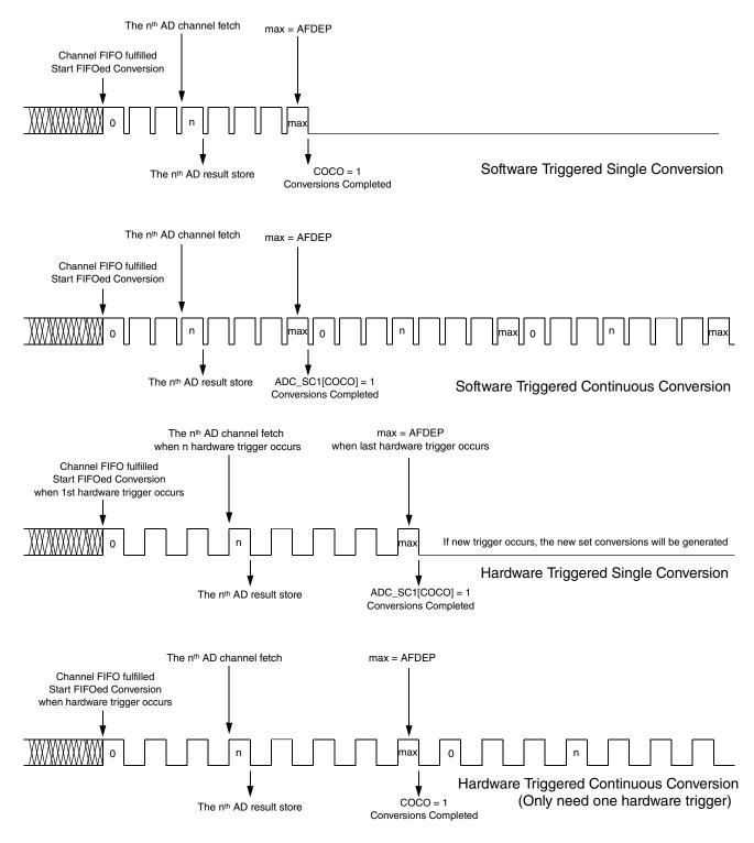
Figure 19-13. ADC FIFO conversion sequence
