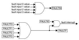
Figure 12-243. FAULTF and FAULTIN bits and fault interrupt
