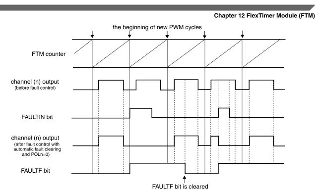
Figure 12-244. Fault control with automatic fault clearing
