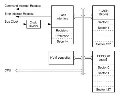
Figure 4-2. Flash and EEPROM block diagram
