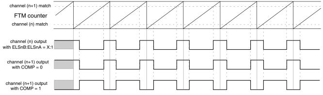
Figure 12-222. Channel (n+1) output in complementary mode with (ELSnB:ELSnA = X:1)
