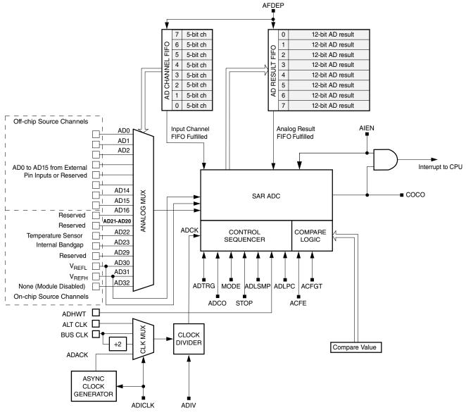
Figure 19-1. ADC Block Diagram
