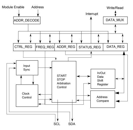
Figure 18-1. I2C Functional block diagram
