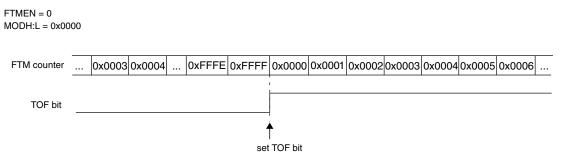
Figure 12-192. Example when the FTM counter is a free running
