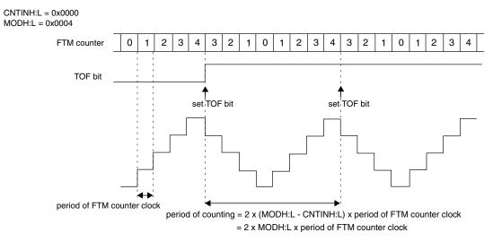
Figure 12-191. Example of up-down counting when CNTIN = 0x0000
