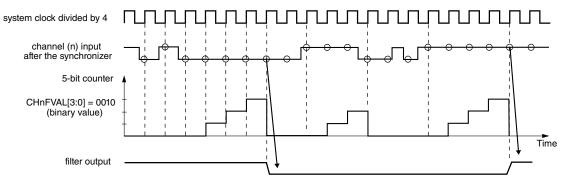
Figure 12-195. Channel input filter example
