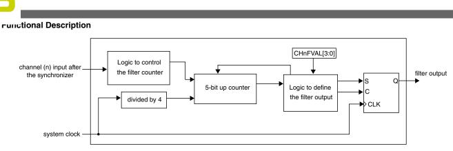
Figure 12-194. Channel input filter
